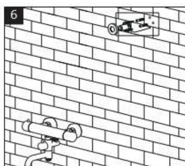
1. Press some silica gel to the gap of wall and the hole. Open the water valve to flush the pipes.
